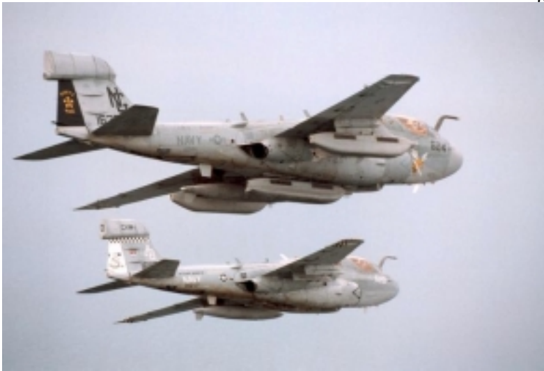
The EA-6B is a joint EW platform that can detect threats, provide standoff jamming, penetrate with a strike package, and shoot HARMs.
