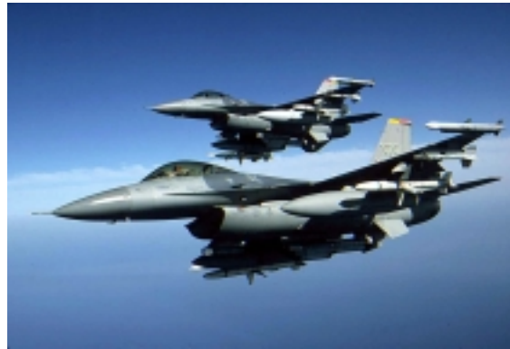
F-16CJ's use a high-speed anti-radiation missile targeting system and missiles to destroy or disable enemy radars.
